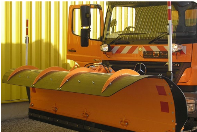
PLOW CAN BE EQUIPPED WITH WHEELS OR SLIDING SKIS
