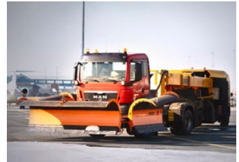
2 FOLDABLE SIDE WINGS FOR EASIER ACCESS TO GARAGE
