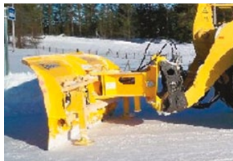
SNOWPLOW WITH FITTING PLATE OR PARALLELOGRAM
