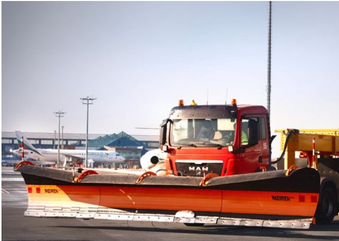
2 FOLDABLE SIDE WINGS FOR EASIER ACCESS TO GARAGE
