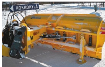
SNOWPLOW WITH FITTING PLATE OR PARALLELOGRAM
