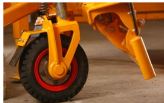
PLOW CAN BE EQUIPPED WITH WHEELS OR SLIDING SKIS
